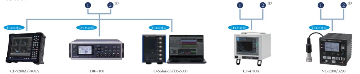
①: 电压输入(CO2型(BNC)接插头) ②: 传感输入(CO2型(BNC)接插头)<sup>注1</sup>
